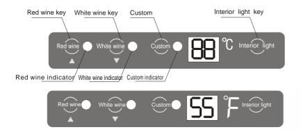
After the power is switched on, all indicators will light up for self-inspection and then the refrigerator will beautomatically set on the redwine mode. Atthat time, the red wine indicator will light up and DISPLAY will show the actual temperature.
